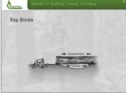
A photograph of a log with a top bind. The log is lying horizontally, and a chain saw is positioned to cut it. The top of the log is labeled 'Compression' and the bottom is labeled 'Tension'.        | <h3>Top Binds</h3> <p><b>Say:</b></p> <p>In top binds, the tension is on the bottom of the log. The compression/bind is on the top.</p> <p><b>INSTRUCTOR NOTE:</b></p> <p>Discuss the example in the image and any experience with top binds that you may have.</p> <p><b>DISPLAY NEXT SLIDE</b></p>
