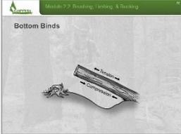
A photograph of a log with a bottom bind. The log is lying horizontally, and a chain saw is positioned to cut it. The top of the log is labeled 'Tension' and the bottom is labeled 'Compression'. | <h3>Bottom Binds</h3> <p><b>Say:</b></p> <p>In bottom binds, the tension is on the top of the log, the compression/bind is on the bottom.</p> <p><b>INSTRUCTOR NOTE:</b></p> <p>Discuss the example in the image and any experience with bottom binds that you may have.</p> <p><b>DISPLAY NEXT SLIDE</b></p>
