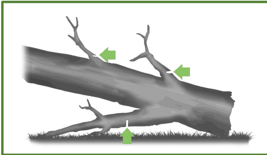
Figure 2.2.3—A tab cut used for limbing.
