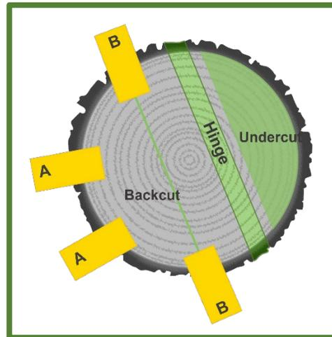
**Figure 2.3.32—Using wedges to move a tree into its objective.**
