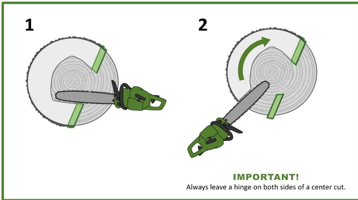
**Figure 2.3.37—Felling cuts for a tree diameter more than twice the length of the chain saw bar.**
