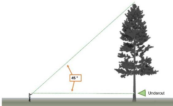
Figure 2.3.1c—Align the stick with the top of the tree and the undercut.
