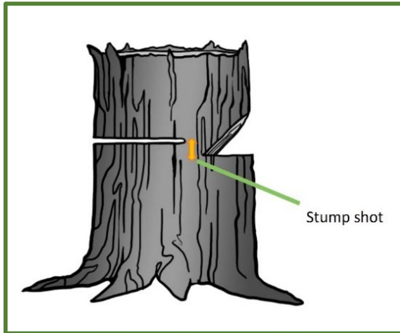
Figure 2.3.22—An example of a step (stump shot).
