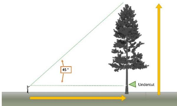
Figure 2.3.1d—The height of the tree is equal to your distance from the tree when you have formed an isosceles triangle.
