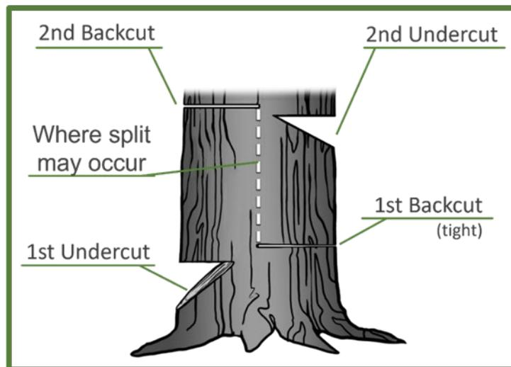
**Figure 2.3.33—Alternative method for a pinched bar.**
