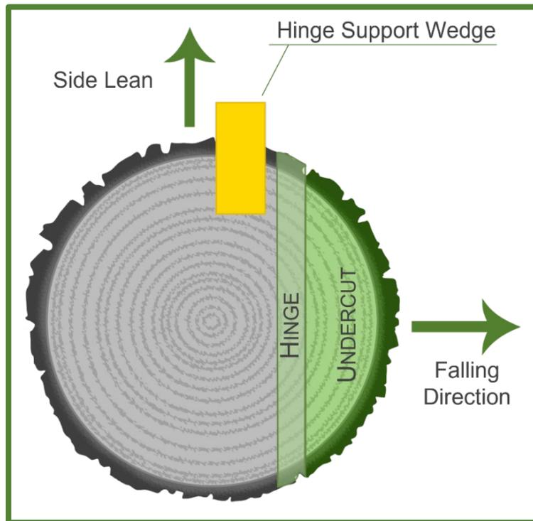
**Figure 2.3.29—Using a stabilizing wedge.**
