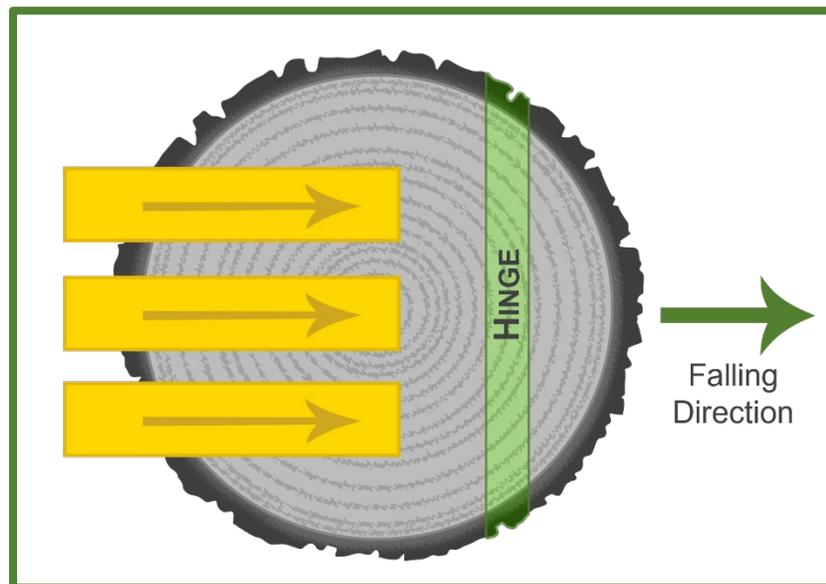
**Figure 2.3.28—Using multiple wedges.**
