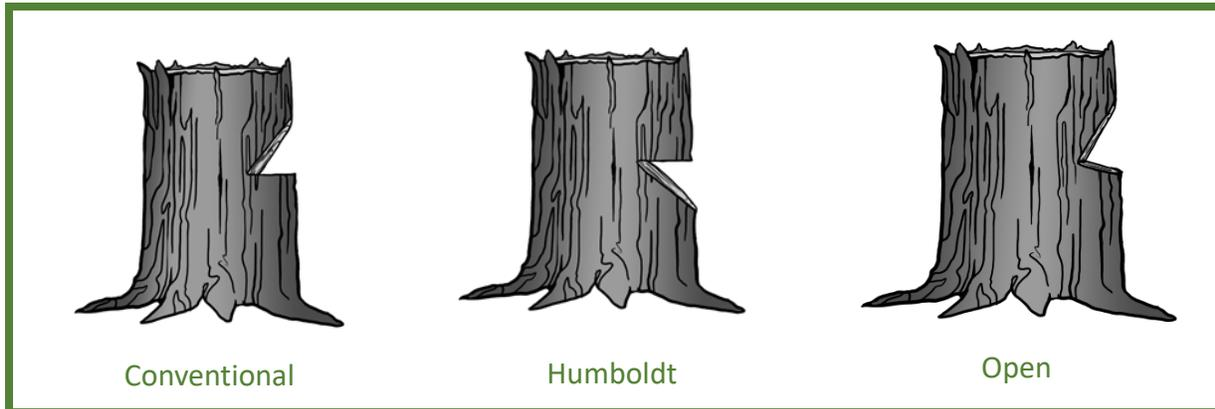
**Figure 2.3.20—Different types of undercut.**
