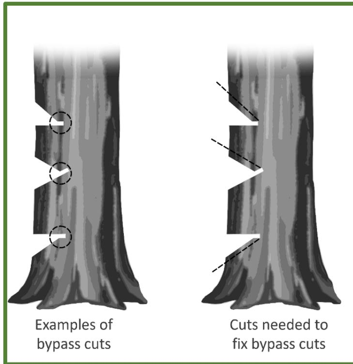
**Figure 2.3.21—Examples of bypass cuts and the cuts required to fix them.**
