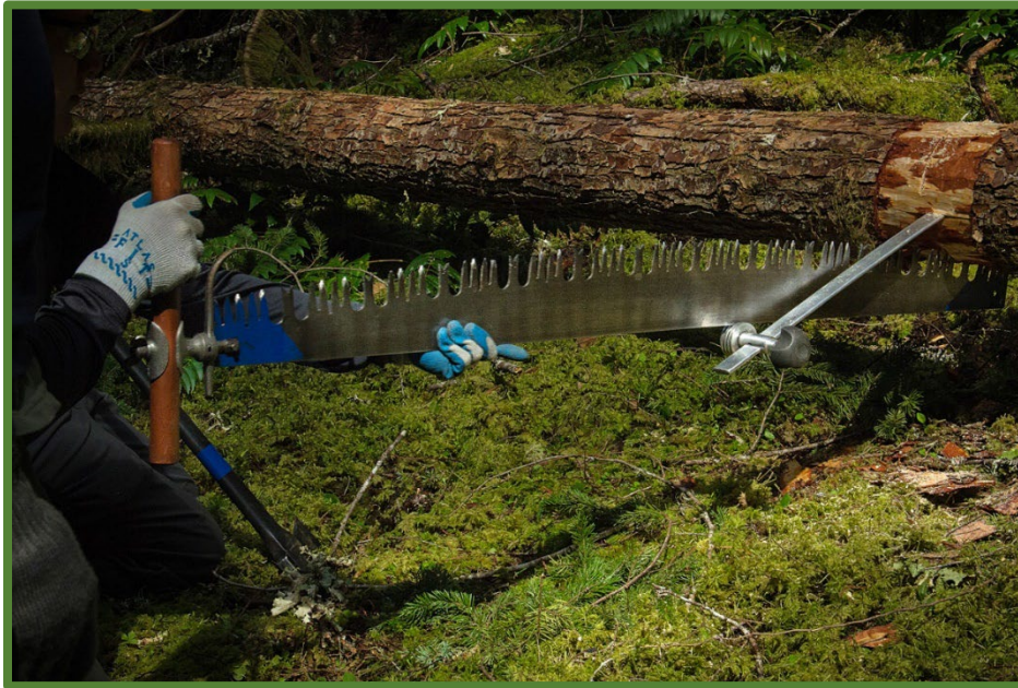
Figure 3.1.22—An underbucker in use.
