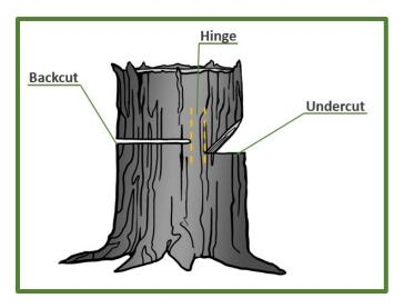
Figure 3.3.18—The anatomy of a hinge.
