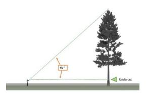
Figure 3.3.2c—Align the stick with the top of the tree and the undercut.
