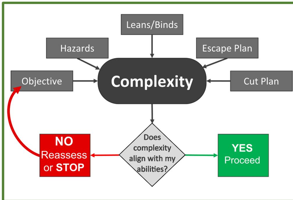
**Figure 3.3.34—The complexity flowchart.**
