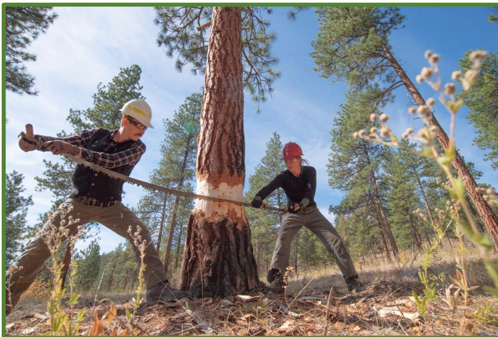
Figure 3.3.28—Proper body position.
