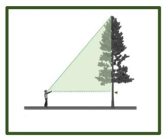
Figure 3.3.2a—Concept for measuring tree height.
