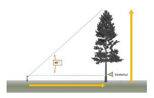
Figure 3.3.2d—The height of the tree is equal to your distance from the tree when you have formed an isosceles triangle.
