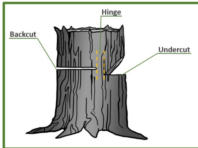
**Figure 3.3.18—The anatomy of a hinge.**
