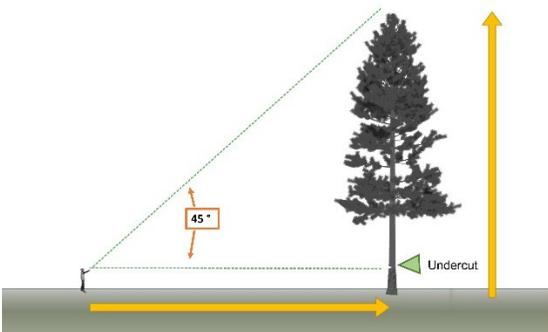
Figure 3.3.2d—The height of the tree is equal to your distance from the tree when you have formed an isosceles triangle.
