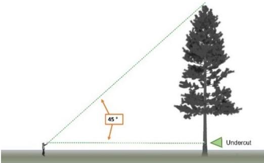
Figure 3.3.2c—Align the stick with the top of the tree and the undercut.
