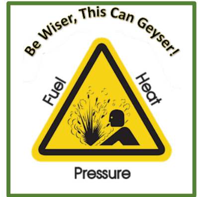
Figure 5.0.1—A fuel geyser warning poster.
