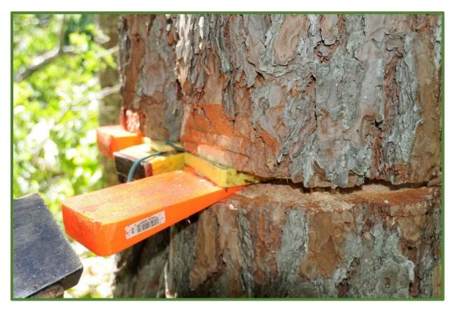
Figure 6.0.14—Combining shims with a standard wedge.
