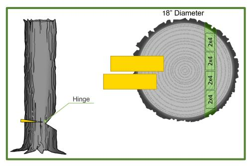
Figure 6.0.16—Elasticity of a hinge.
