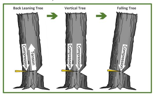
Figure 6.0.15—Tensile strength.
