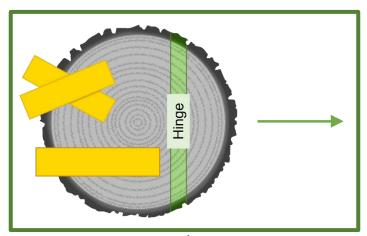
Figure 6.0.13—Crossing/stacking wedges.
