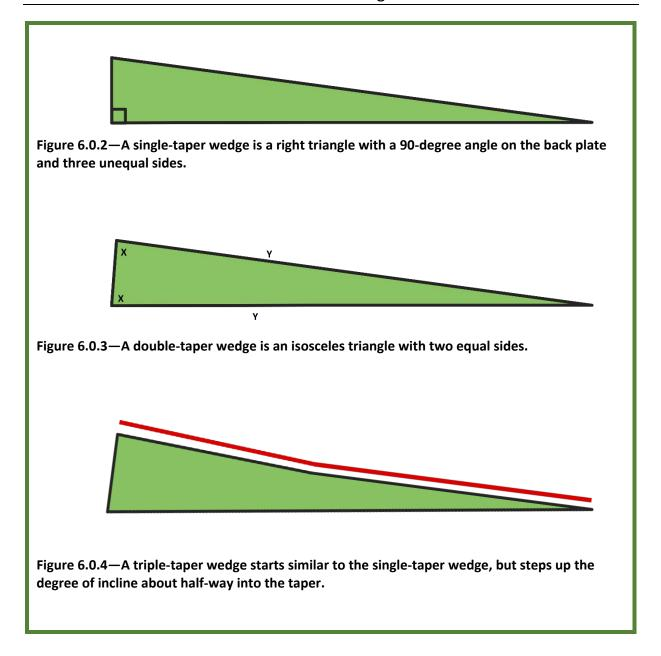
Note: The triple-taper wedge works well for quicker lift on smaller trees. On heavier, larger trees, it lifts slowly to get the action started and then a quicker lift takes over. Because of the drastic change in taper, a triple-taper wedge is more difficult to drive toward the back of the wedge.
