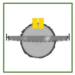
Figure 6.0.9—Wedging technique for top bind.
