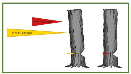
Figure 6.0.1—Calculating mechanical advantage.
